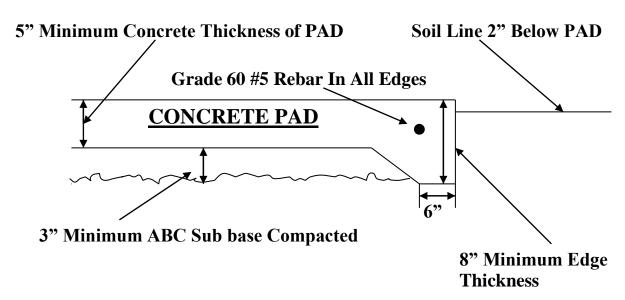
Minimum 3000# PSI Concrete Mix Slump not to exceed 4.5"
